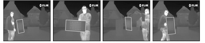
Fig. 4: Boundary of the calibration board projected into the IR images based on the automatically calibrated intrinsic and extrinsic IR camera parameters.
